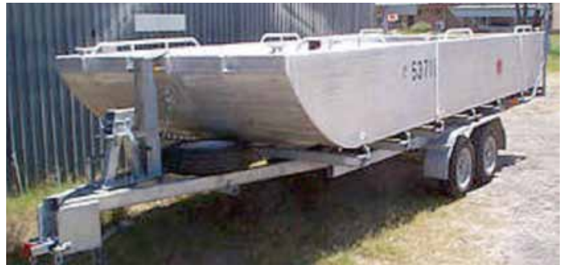
6 meter aluminium work boat made to order for the National Parks and Wildlife Service
